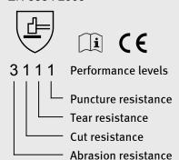
Pictogram and performance levels according to EN 388:2003 (highest performance level: 4/cut resistance:
