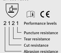
Pictogram and performance levels according to EN 388:2003 (highest performance level: 4/cut resistance:
